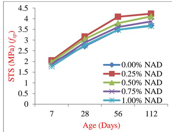
Figure 10.D. Splitting tensile strength of C-55\_FA-45
