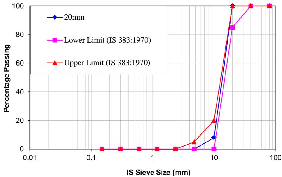
Figure 2. Grading curve of 20 mm coarse aggregate
