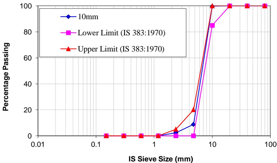
Figure 3. Grading curve of 10 mm coarse aggregate
