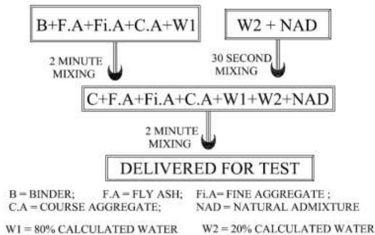
**Figure5. Mixing process of concrete ingredients**
