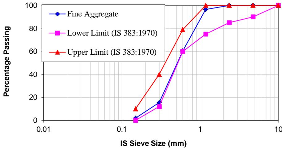
Figure 4. Grading curve of fine aggregate
