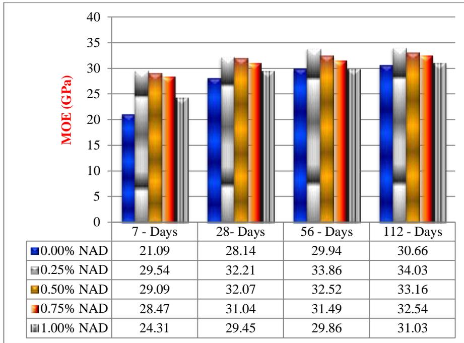
Figure 11.A. Modulus of Elasticity of C-100\_FA-0
