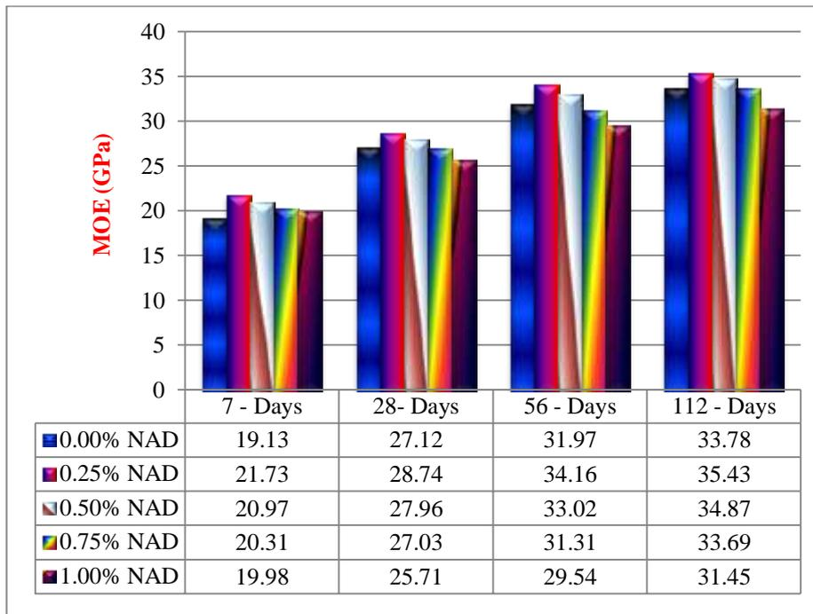
Figure 11.C. Modulus of Elasticity of C-65\_FA-35
