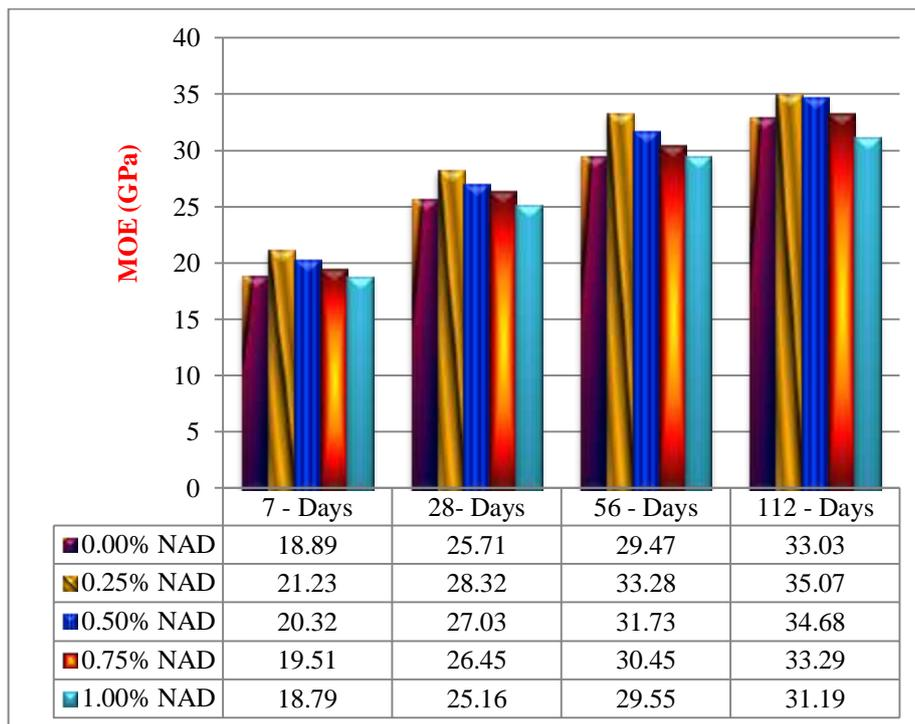
Figure 11.D. Modulus of Elasticity of C-55\_FA-45
