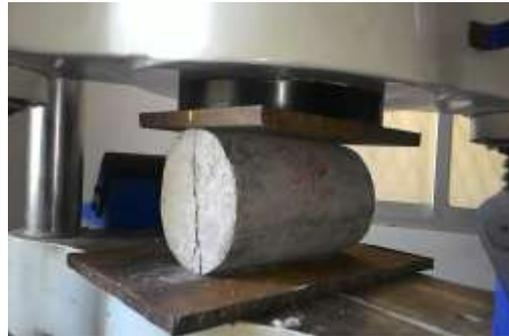
Figure 7. Splitting tensile failure of cylinder
