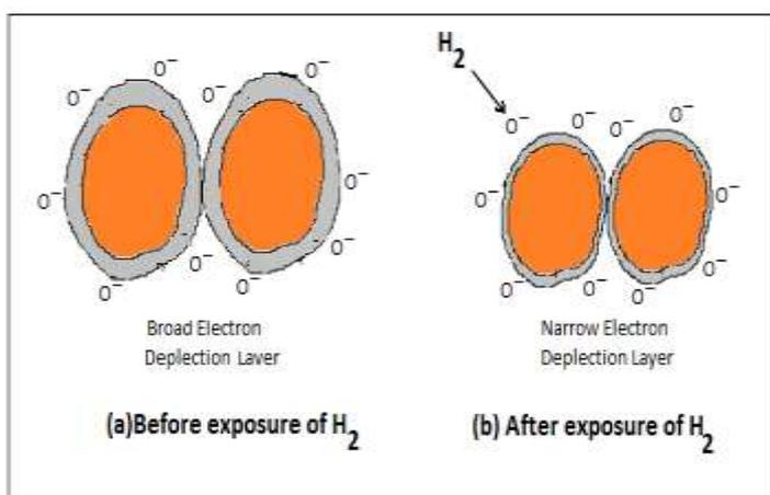
**Fig 7: Sensing mechanism of  $\text{ZnSnO}_3$  thin film**
