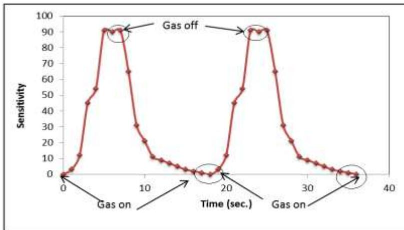
**Fig. 6: Response and recovery profile of the sensor.**
