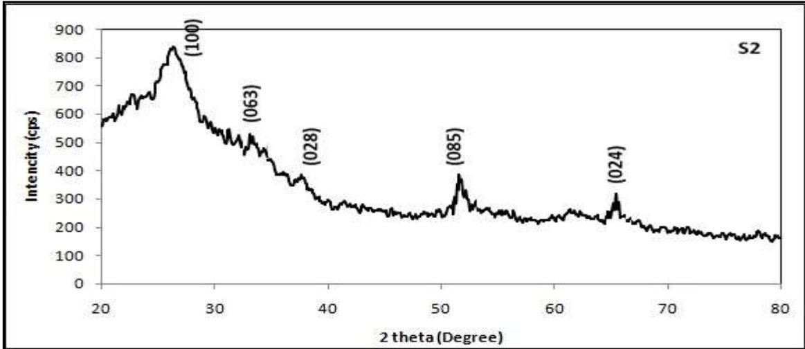
**Fig 1: X-ray diffractogram of most sensitive nanocrystalline ZnSnO<sub>3</sub> thin film sample S2.**
