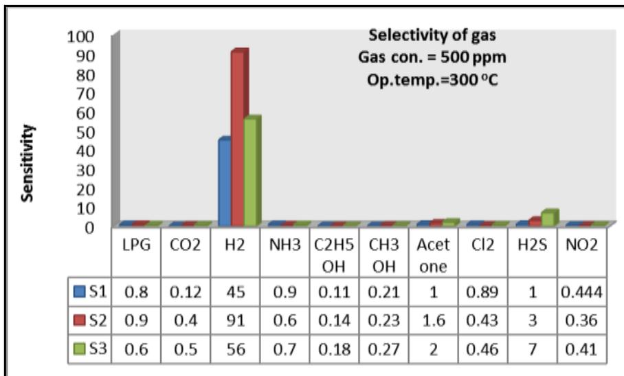
Fig. 5: Selectivity profile against various tested gases.
