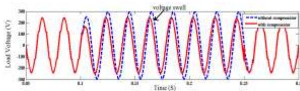
**Fig.11.** Load voltage with and without compensator under nonlinear load with PI controller
