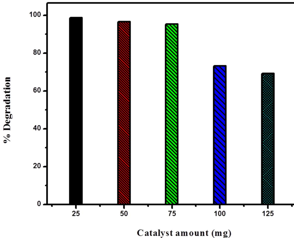
Fig9.Effect of catalyst loading, [MB]= $10^{-5}$  mol L<sup>-1</sup>, catalyst used =3 wt% Ag-ZnO, pH = 11 irradiation time = 120 min.
