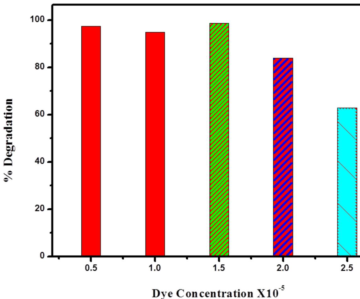
**Fig10.** The effect of initial concentration of MB on irradiation with LED light in the presence 3% Ag-ZnO; pH = 11 catalyst suspension =  $0.50 \text{ gL}^{-1}$  at different initial concentration.
