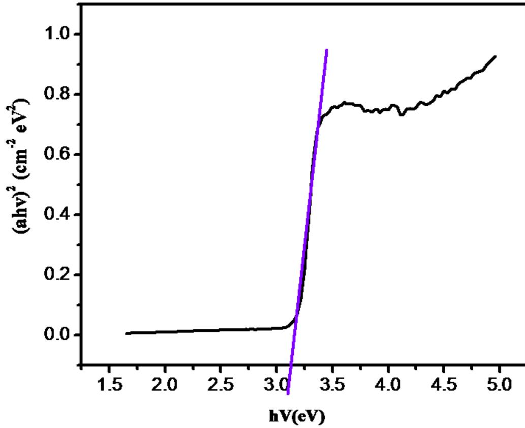
Fig5. Plot for band-gap energy ( $E_{bg}$ ) of Ag-ZnO
