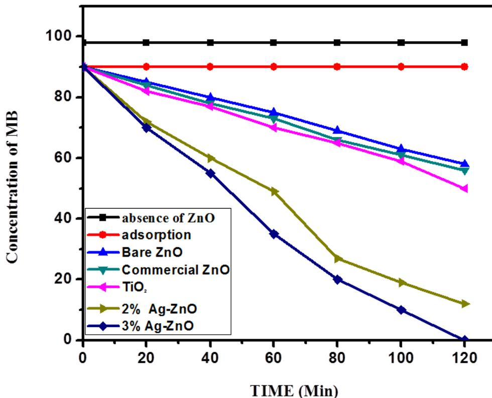
**Fig7.** Photodegradability of MB; dye concentration =  $10^{-5}$  mol L<sup>-1</sup> Catalyst suspension = 0.5 g L<sup>-1</sup>, pH = 11 with ZnO bare and Ag doped ZnO Catalyst.
