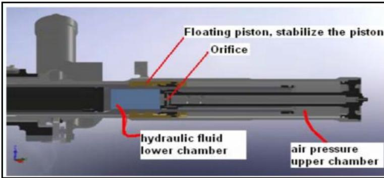
**Fig 3 Shock Absorber cross section**
