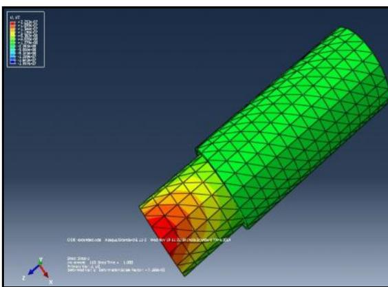
**Fig 4. Deflection in oleo shock absorber**
