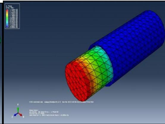
**Fig 5. Von mises stress in oleo shock absorber**
