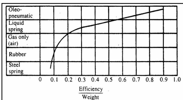
Fig 1 Shock absorber efficiency
