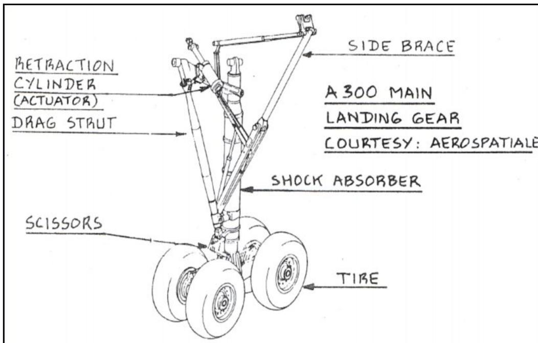
**Fig 2 Example of shock absorber and tyre**
