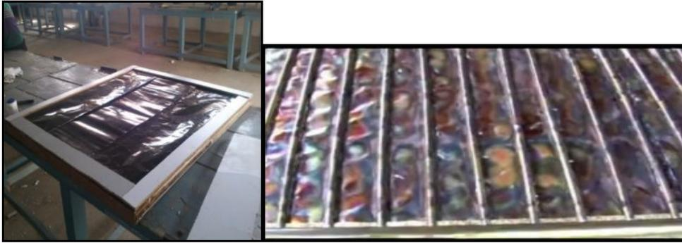
**Fig 3. Flat-Plate Collector**
