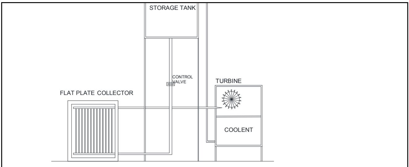
**Fig 7 Components arrangements for solar power generation**
