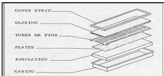
**Fig 4. component arrangement**
