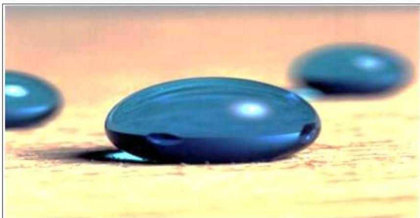
**Figure 3: A hydrophobic wooden surface. BASF AG**
