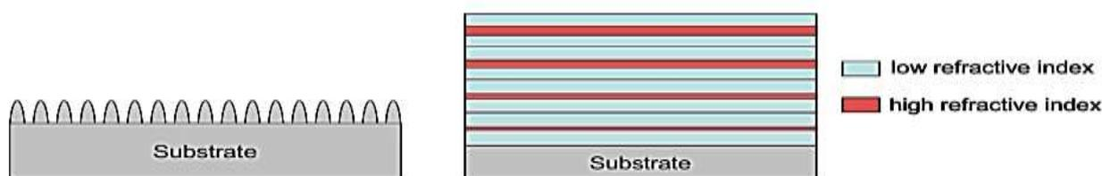
**Figure 6: Comparison between a moth-eye structured surface (left) and an antireflective coating(right). Both methods reduce the reflection efficiently.**
