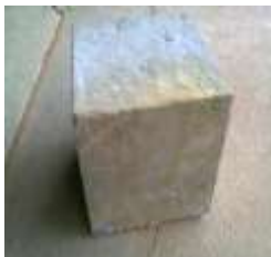
Figure .2 Concrete cube subjected to sulphate attack
