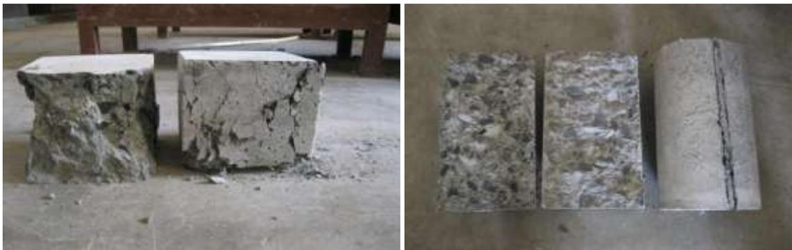
**Figure 3:- Ductile behaviour of compressive strength specimen(left) and tensile strength specimen (right) with and without PET fibers( Nibudey et.al 2013)<sup>15</sup>**
