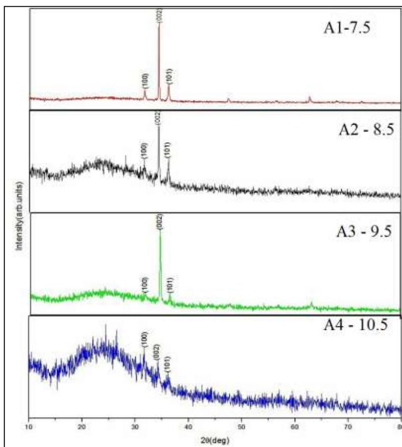
**Figure 1 XRD Spectra of different pH values of 7.5, 8.5, 9.5 and 10.5.**
