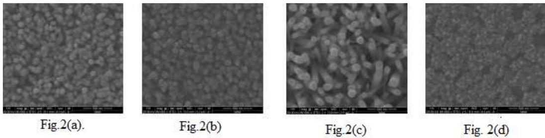
**Figure 2. SEM pictures of ZnO nanorods of different pH values of 7.5, 8.5, 9.5 and 10.5.**
