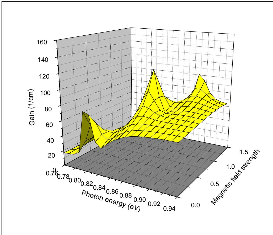
**Figure 1.** Variation of gain as a function of photon energy for various values of measure of magnetic field strength in a  $\text{InAs}_{0.8}\text{P}_{0.2}/\text{InP}$  quantum well wire with the constant electron density
