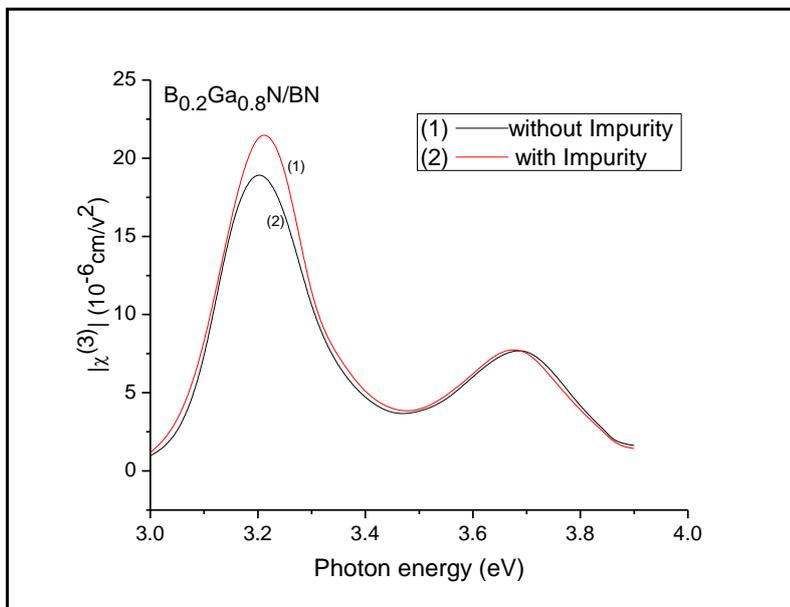
**Figure1. Variation of third-order susceptibility of third harmonic generation as a function of incident photon energy in a  $B_xGa_{1-x}N/BN$  quantum well**
