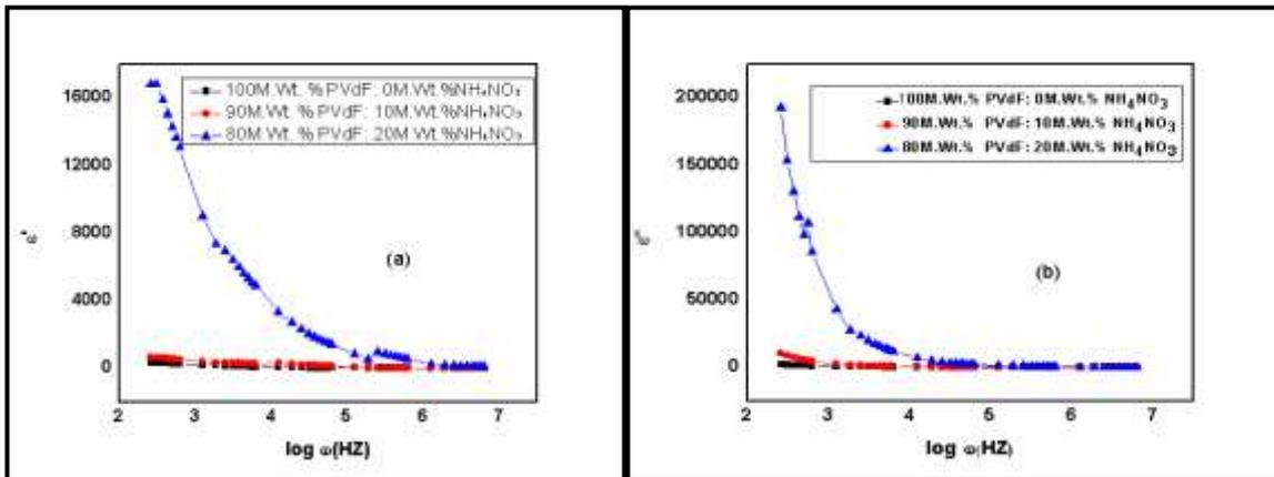
**Figure 3** Frequency dependence of (a)  $\epsilon'(\omega)$  for x PVdF : (1-x)  $\text{NH}_4\text{NO}_3$  systems Frequency dependence of (b)  $\epsilon''(\omega)$  for x PVdF : (1-x)  $\text{NH}_4\text{NO}_3$  systems at room temperature.
