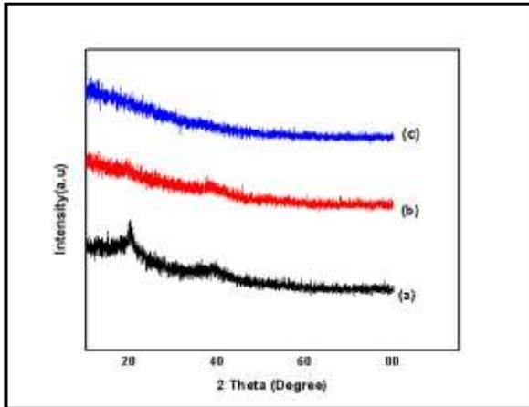
**Figure 1** XRD patterns of (a) Pure PVdF, (b) 90 PVdF: 10  $\text{NH}_4\text{NO}_3$ , (c) 80 PVdF: 20  $\text{NH}_4\text{NO}_3$
