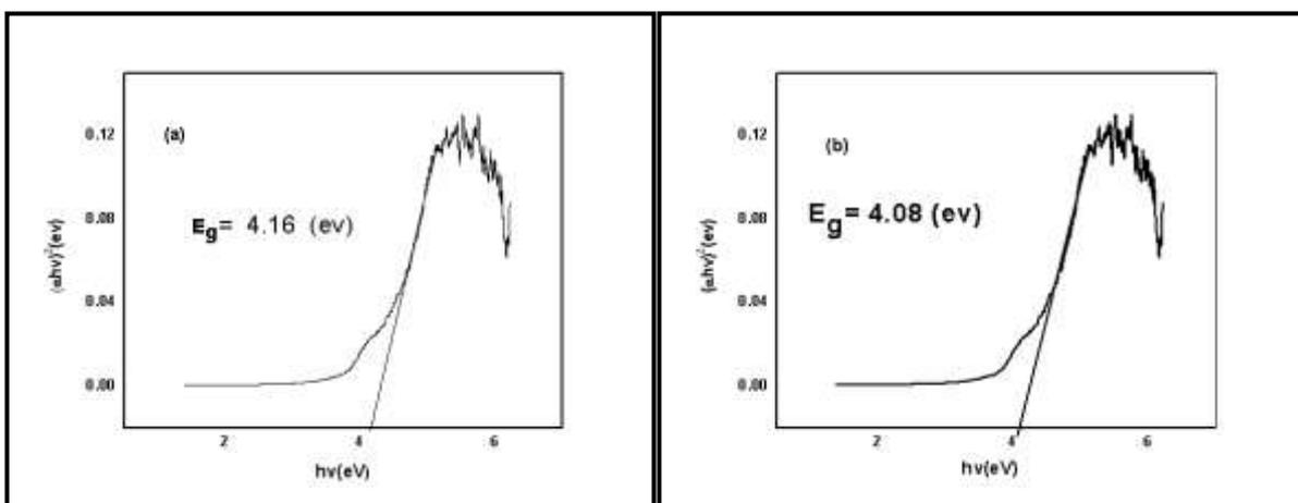
**Figure 4** (a) (b) UV-visible spectra for pure PVdF and 80%PVdF: 20% $\text{NH}_4\text{NO}_3$ .
