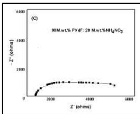
Figure 2 (a) (b) (c) show the complex impedance plot for x PVdF:(1-x) NH<sub>4</sub>NO<sub>3</sub> polymer Electrolyte systems at ambient temperature (303K).
