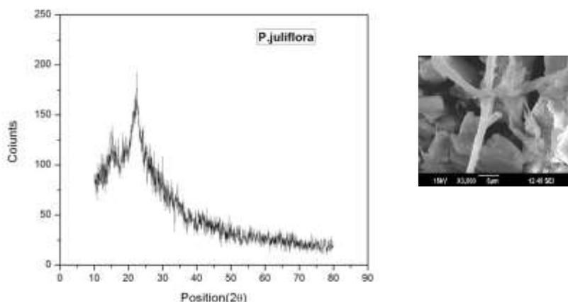
Fig.1. Room temperature XRD pattern and SEM micrograph of *P.juliflora*
