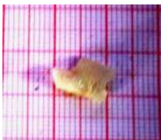
Fig. 2 Photograph of GGLY Crystal grown from \alpha Glycine and 4-Chlorobenzoic acid
