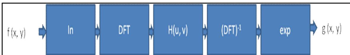
**Fig. 1 Steps in homomorphic filtering**
