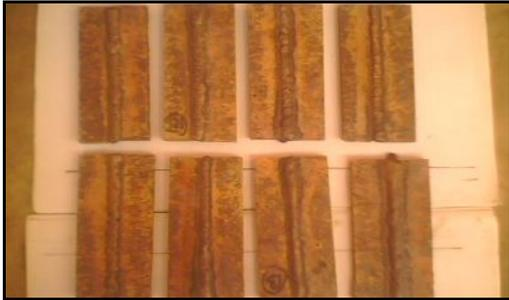
Fig. 2.1. TIG Welding specimen
