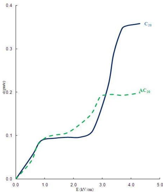
**Fig. 3 Dc-field dependence of the effective second order susceptibility for the  $\text{Li}_2\text{O-ZrO}_2\text{-SiO}_2$  glasses doped with 0.20 mol % of CuO before and after crystallization**
