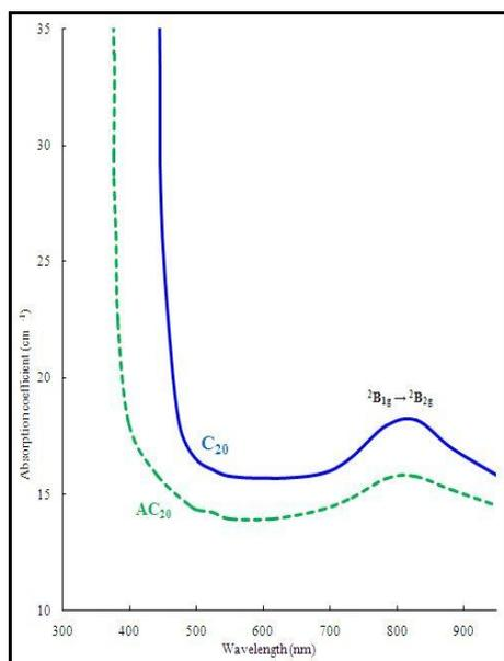
**Fig. 1 Optical absorption spectra of  $\text{Li}_2\text{O}-\text{ZrO}_2-\text{SiO}_2$  glasses doped with 0.20 mol % of CuO recorded at room temperature before and after crystallization**
