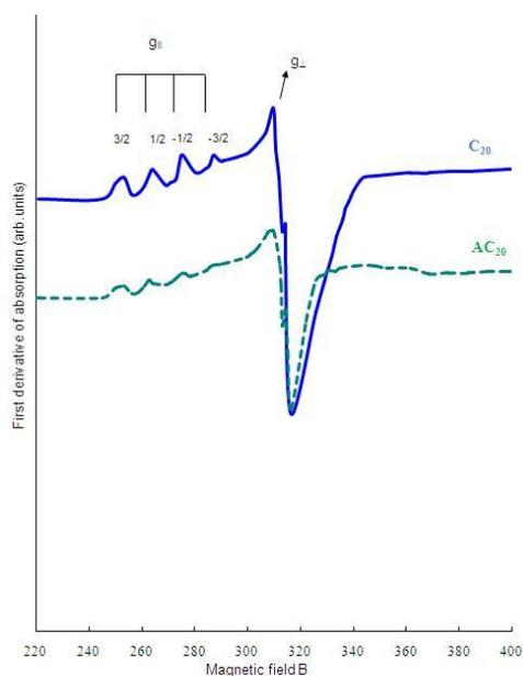
**Fig. 2 ESR spectra of  $\text{Li}_2\text{O}-\text{ZrO}_2-\text{SiO}_2$  glasses doped with 0.20 mol % of CuO recorded at room temperature before and after crystallization**
