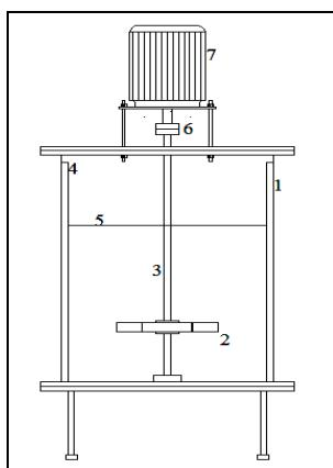
**Figure:1 Gas inducing mechanically agitated contactor**
