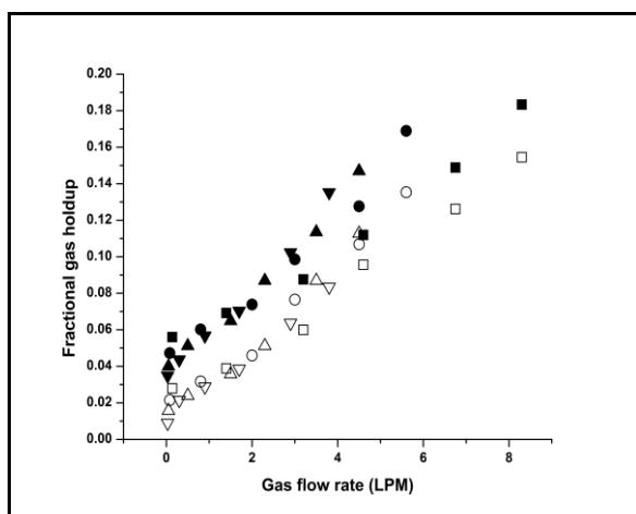
**Figure 8 - Relation between fractional gas holdup with gas flow rate at various immersion depths of 20cm (□)sparging and (■)induction, 25cm (○)sparging and (●)induction, 30cm (△)sparging and (▲)induction and 35cm (▽)sparging and (▼)induction.**
