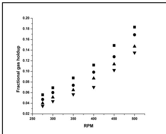
**Figure 7 - Relation between the gas holdup and rotational speed at various submersion depths of (■)20cm, (●)25cm, (▼)30cm, (▲)35cm**
