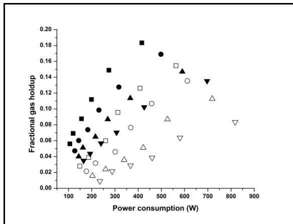
**Figure 7 - Relation between fractional gas holdup and power consumption at various immersion depths of 20cm (□)sparging and (■)induction, 25cm (○)sparging and (●)induction, 30cm (△) sparging and (▲)induction, and 35cm (▽)sparging and (▼)induction.**
