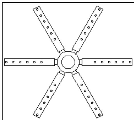
**Figure 3: Top view of the hollow turbine impeller**
