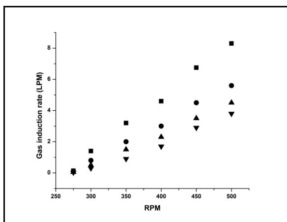
**Figure 4- Effect rotational speed on gas induction rate for different impeller immersion depths of (■)20cm, (●)25cm, (▲) 30cm and (▼)35cm**
